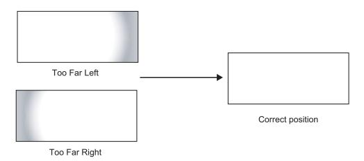
4. When the horizontal position is properly set, tighten the Yaw/X-Adjustment Levers to secure the lens in place.
